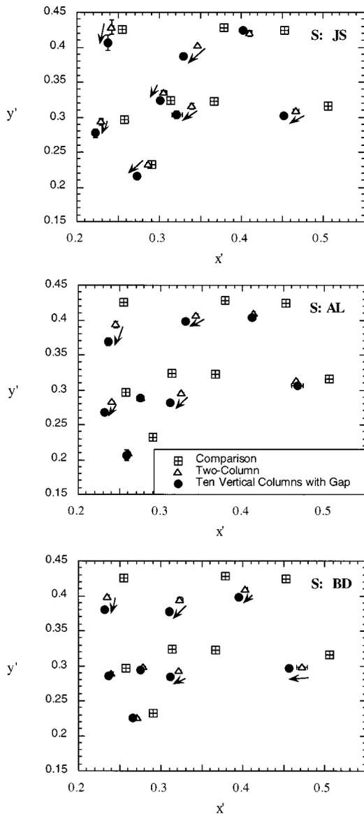
Fig. 6. Hue and saturation matches (in Judd space) for the two-column uniform vertical surrounds (triangles) and the ten-column vertical surround with a 2° dark gap (circles).
