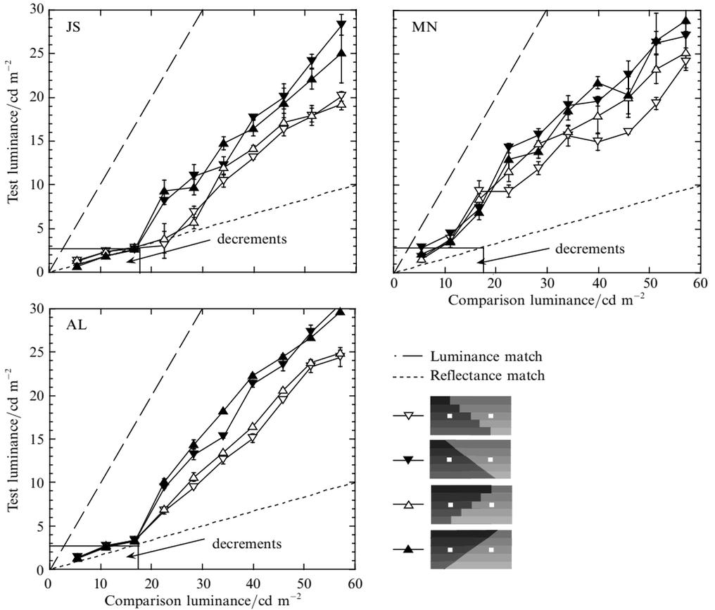
**Figure 6.** Brightness matches made on horizontal stripes with a stair-step edge (open triangles) or with a straight angled edge (filled triangles). Only the latter is an apparent illumination edge.
